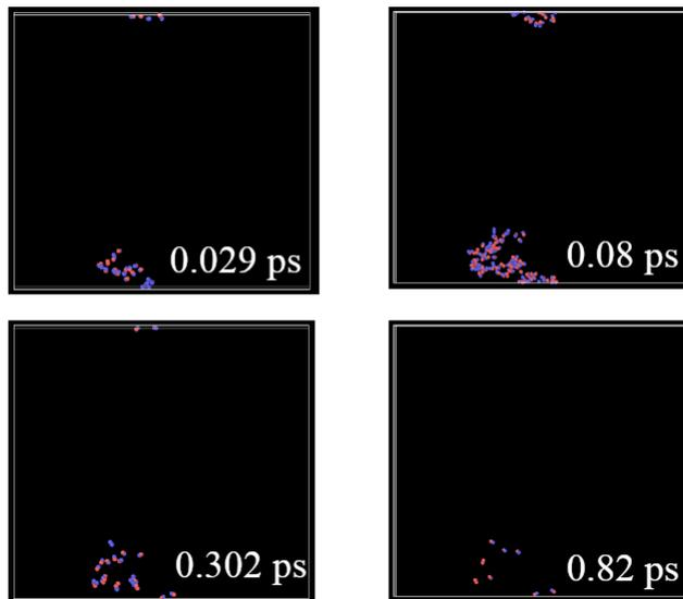
These are taken in chronological order and show the total defects at different points in time. As is to be expected, at the very beginning defects very quickly form as the knock-on atom deposits almost all of it's kinetic energy at once. This causes the radiation cascade to begin forming, and ballooning outward from where the knock-on atom first struck the lattice. Of note is that as the knock-on atom recoils from it's first
