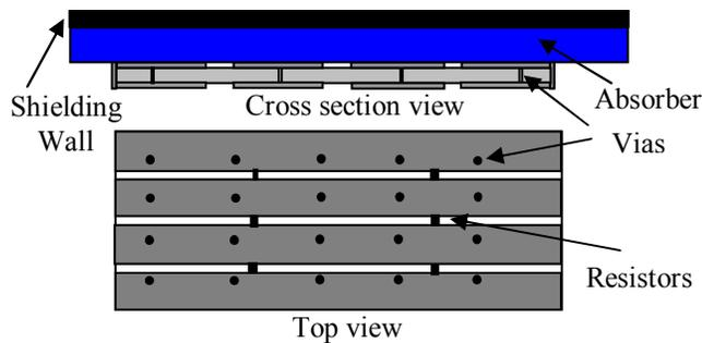
Figure 5. PCB walls of the modified TEM cell.
