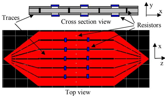
Figure 4. PCB septum of the modified TEM cell.
