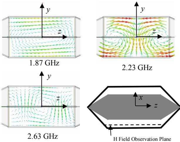
Figure 2. Longitudinal magnetic field ( $H_z$ ) at resonant frequencies.
