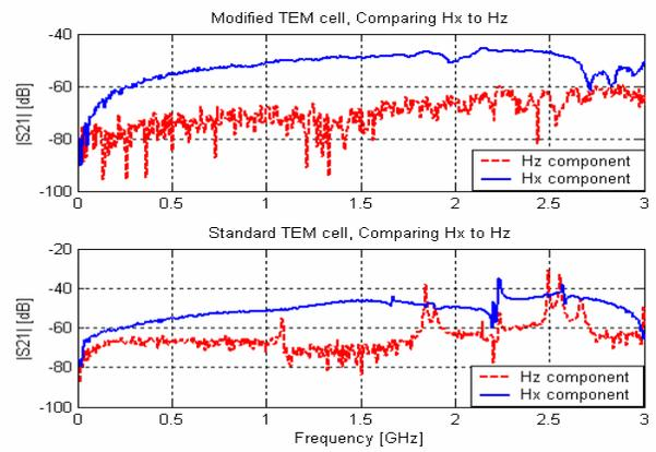
Figure 16. Ratio of  $H_z$  to  $H_x$  (main component)
