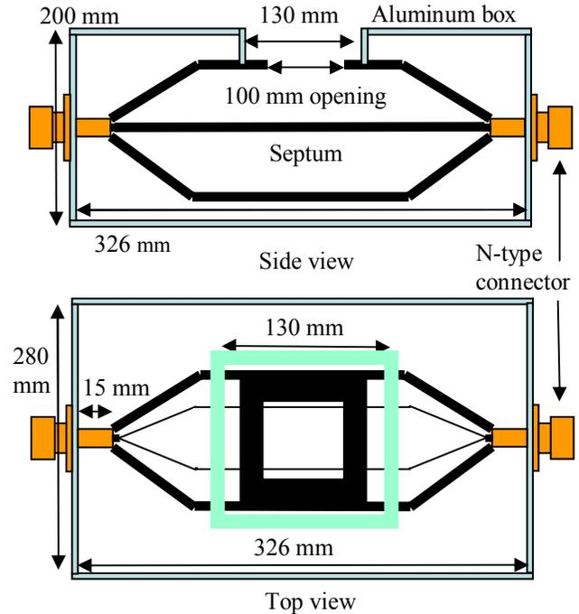
Figure 3. Geometry of the modified TEM cell.
