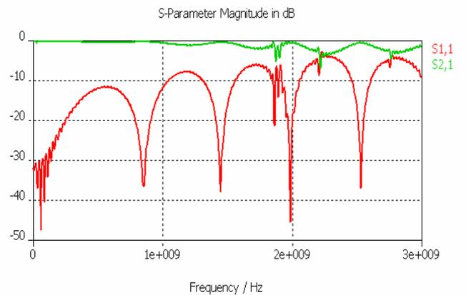
Figure 7. Simulated S parameters for open parallel-trace cell.
