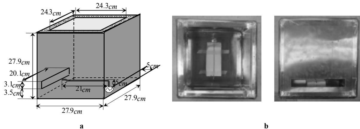
Fig 2. (a) Geometry data of wire and semi-open box; (b) Experimental model of the semi-open box
