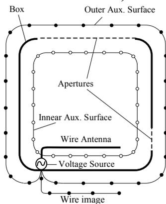
**Fig 1. The model of the box with openings**
