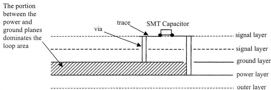
Fig. 6. Current loop for an SMT decoupling capacitor.
