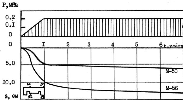
Fig. 1. Time-settlement curves for a 5-storey building on strip foundation.
