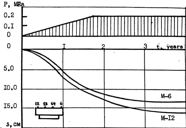
Fig. 2. Time-settlement curves for a 9-storey building on raft foundation.
