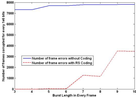
Fig. 7. Comparison of the Number of Correct Frames Received
