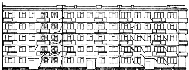
Fig.4. State of the front wall cracks till the general renovation and applied protections
