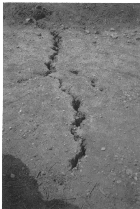
Fig. 5. Shrinkage Cracks on the Ground Surface
