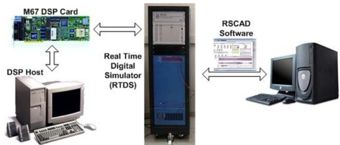
Figure 6. Experimental setup block diagram.
