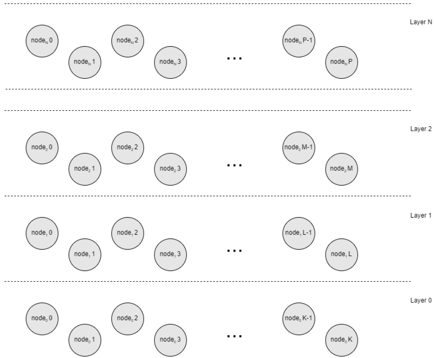
Fig. 2. Multilayered Peer-to-Peer network and layered nodes
