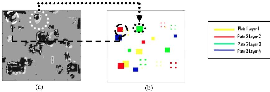
**FIGURE 5.** Data fusion results (a) multimodal fusion Image, (b) schematic of the stack of corroded panels.
