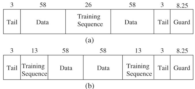
Fig. 2. (a) Original EDGE slot structure. (b) Slightly modified slot structure.
