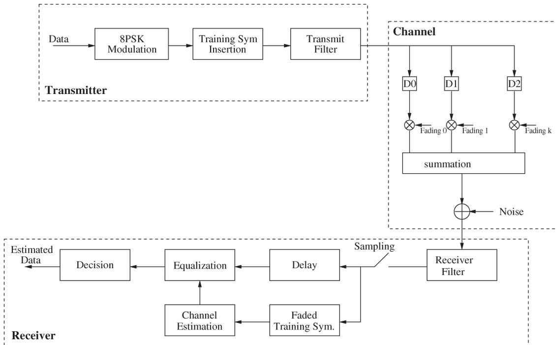
Fig. 1. Block diagram of the baseband EDGE system.
