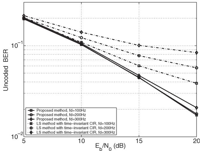
Fig. 7. BER of LS and proposed channel-estimation algorithm employing the DDFSE ( $K = 2$ ) equalizer at  $f_d = 100, 200,$  and  $300$  Hz in HT profile.
