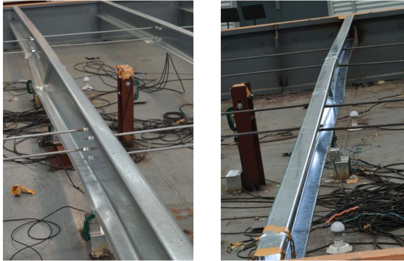
Figure 7. Failure modes of Z-purlin and C-purlin with two rows of sag rods
