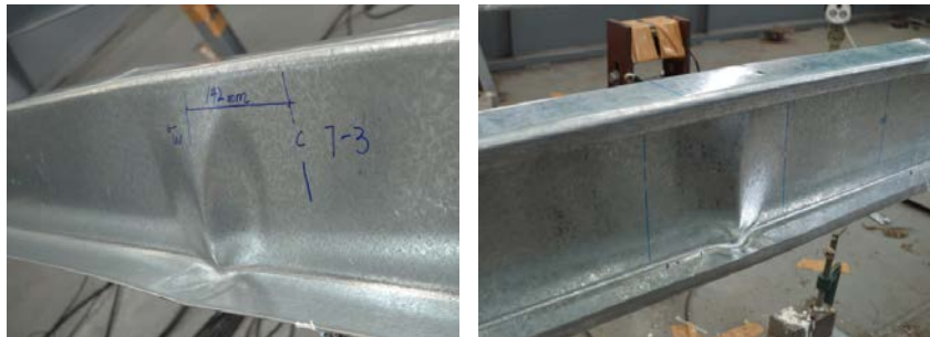
(b) Local buckling of Z-purlin and C-purlin
