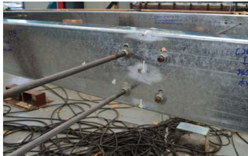
Figure 3. Sag rod configuration
