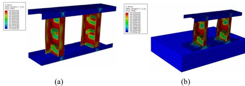
Figure 3: 3D view of deformed stud-track assembly under the peak loads; (a) rigid bearing condition, (b) 1 inch edge distance condition
