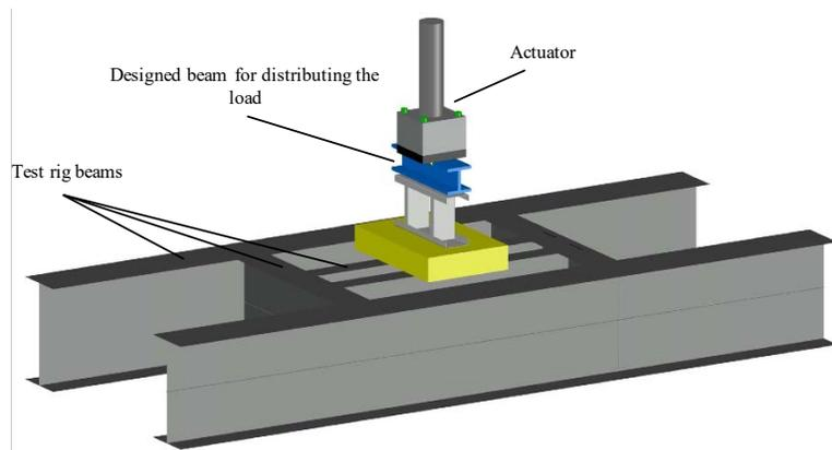
Figure 6: The schematic view of experiment tests
