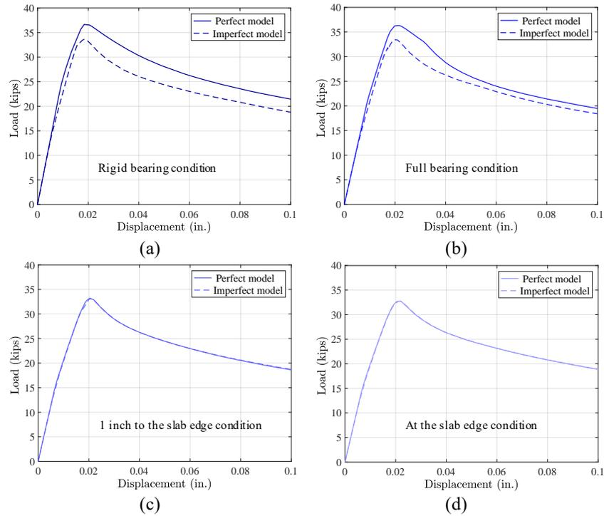
Figure 5: Comparison between the behavior of perfect and imperfect models; (a) rigid bearing condition, (b) full bearing condition, (c) 1 inch to the slab edge condition, (d) at the slab edge condition
