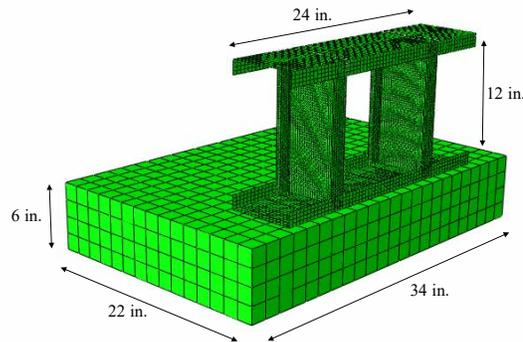
Figure 2: Finite element model of stud-track assembly placed on top of a concrete slab with 1 inch edge distance; the studs are 600S162-54 and the tracks are 600T125-54
