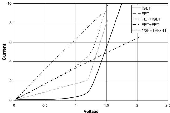
Fig. 1: Forward Characteristics of Various Device Configurations
