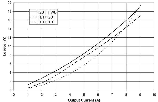
Fig. 7: Experimental Results, Actual Power Loss, 70% Duty Cycle
