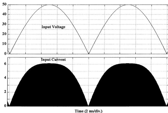
Fig. 7. Input voltage and current in PFC application.
