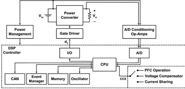
Fig. 3. Block diagram of the digital current controller.
