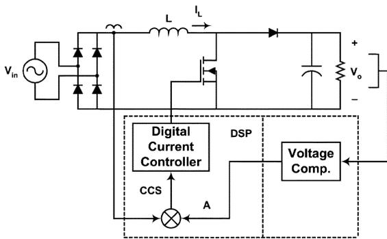
Fig. 6. Block diagram of the PFC converter.
