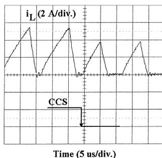
Fig. 8. Inductor current transient response to a step down change in CCS.
