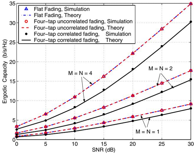
Fig. 1. Ergodic Capacity vs SNR for the SISO,  $2 \times 2$  and  $4 \times 4$  systems over: 1) spatially-uncorrelated frequency flat fading channel; 2) spatially-uncorrelated frequency-selective four-tap-uncorrelated fading channel; 3) spatially-uncorrelated frequency-selective four-tap-correlated fading channel with  $\Psi_{ISI}(i, j) = \frac{0.95^{|i-j|}}{4}$ .
