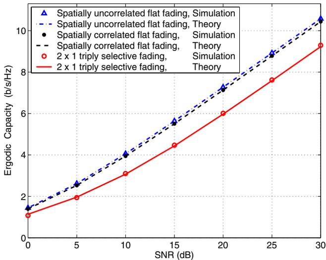
Fig. 2. Ergodic Capacity vs SNR for a  $2 \times 1$  system over: 1) spatially-uncorrelated frequency flat fading; 2) spatially-correlated frequency flat fading with  $\Psi_{RX} = [1 \ 0.7; \ 0.7 \ 1]$ ; 3) triply selective fading with  $\Psi_{RX} = [1 \ 0.7; \ 0.7 \ 1]$  and  $\Psi_{ISI}(i, j) = \frac{0.95^{|i-j|}}{4}$ .
