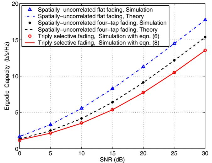
Fig. 3. Ergodic Capacity vs SNR for a  $2 \times 2$  system over: 1) spatially-uncorrelated frequency flat fading; 2) spatially-uncorrelated frequency-selective fading with  $\Psi_{ISI}(i, j) = \frac{0.95^{|i-j|}}{4}$ ; 3) triply selective fading with  $\Psi_{TX} = [1 \ 0.7; \ 0.7 \ 1]$ ,  $\Psi_{RX} = [1 \ 0.7; \ 0.7 \ 1]$  and  $\Psi_{ISI}(i, j) = \frac{0.95^{|i-j|}}{4}$ .
