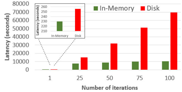
FIGURE 18. Iterative querying performance of in-memory and disk caching engines for one-million smart meters in 4-nodes cluster.
