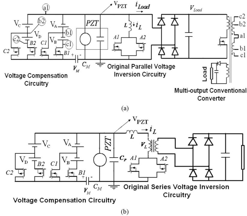
Fig. 2. (a) Parallel voltage compensation topology. (b) Series voltage compensation topology [14]. The capacitor  $C_M$  is added for measuring the transferred charge to PZT in compensating stages and is not part of the topology.
