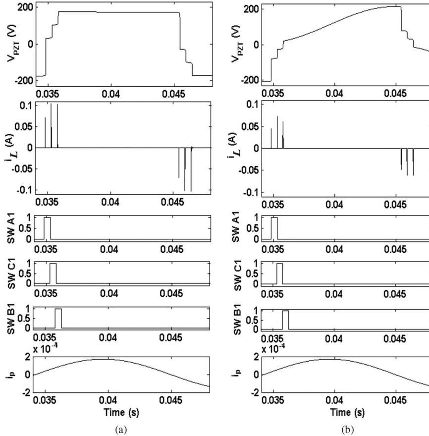
Fig. 4. Voltage and current waveforms. (a) Parallel voltage compensation topology. (b) Series voltage compensation topology. Pulse durations are bigger than those of lab tests for better graph quality.
