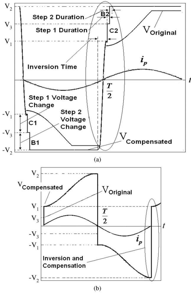
Fig. 3. (a) PZT voltage  $V_{PZT}$  waveforms in the original parallel voltage inversion technique and in voltage compensation scheme with two-step compensation. (b) Voltage levels in series voltage compensation scheme.
