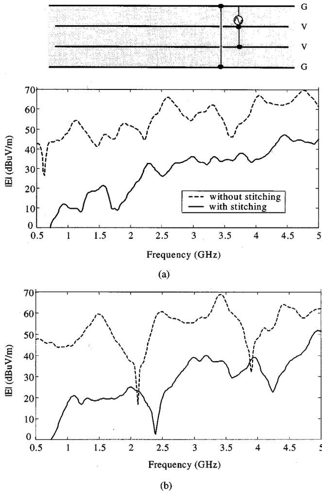
Fig. 14. Modeled EMI at 3 m for the cases with and without stitching for the GVVG configuration with a source placed in between planes. (a)  $E_x$  polarization. (b)  $E_y$  polarization.
