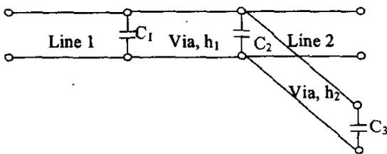
Figure 3. An equivalent circuit for the geometry shown in Fig. 2.
