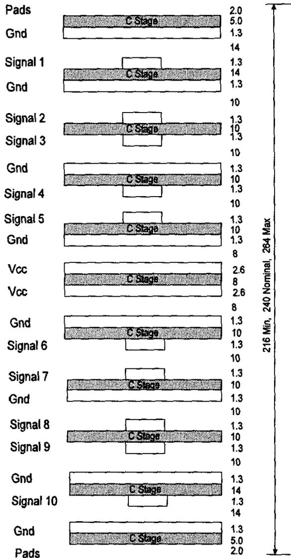
Figure 7. A typical layer stackup for backpanels.
