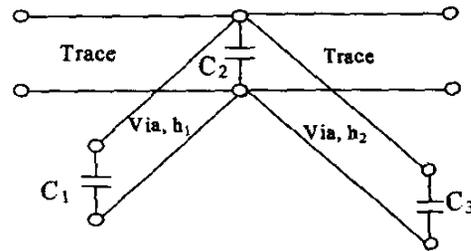
Figure 8. An equivalent circuit for the validation geometry.
