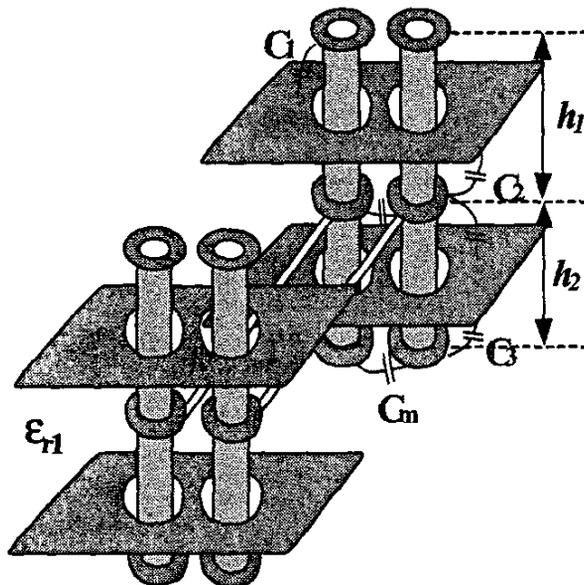
Figure 11. Differential signaling in backpanel with PTH vias.
