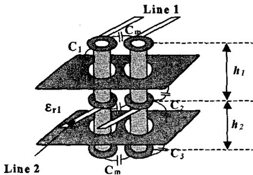
Figure 4. Example geometry: a differential case.
