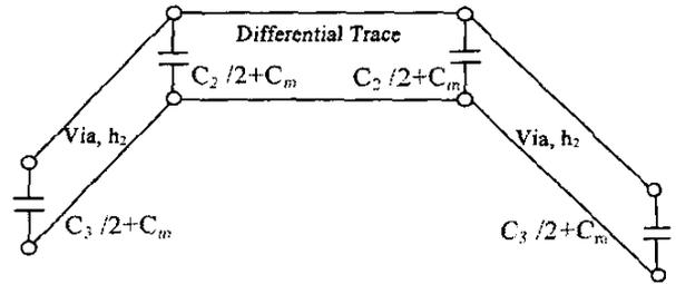
Figure 12. Equivalent lumped circuit for the differential signaling.
