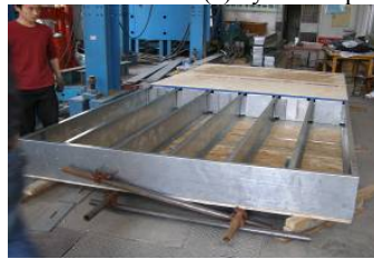
(b) Steel skeleton of specimen FL-1
