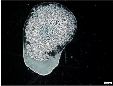
**Figure 9—SiO<sub>2</sub> drop on glass. The bar shown is 1000 μm. Initial concentration of silica is 0.40 weight fraction.**
