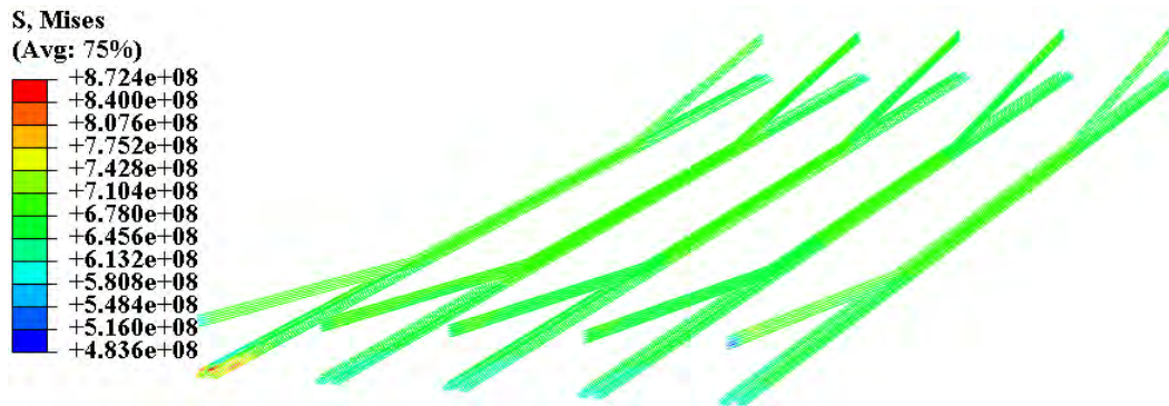
Fig. 3.9 Von Mises stress in prestressed tendons. ( \times 10 ).
