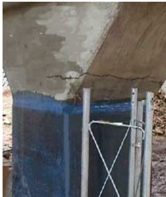
Figure 4.13. Crack at failure of column B2P2.
