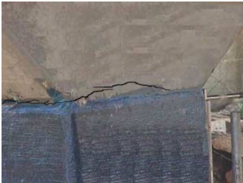
Figure 4.33. Crack at column/haunch intersection at failure.
