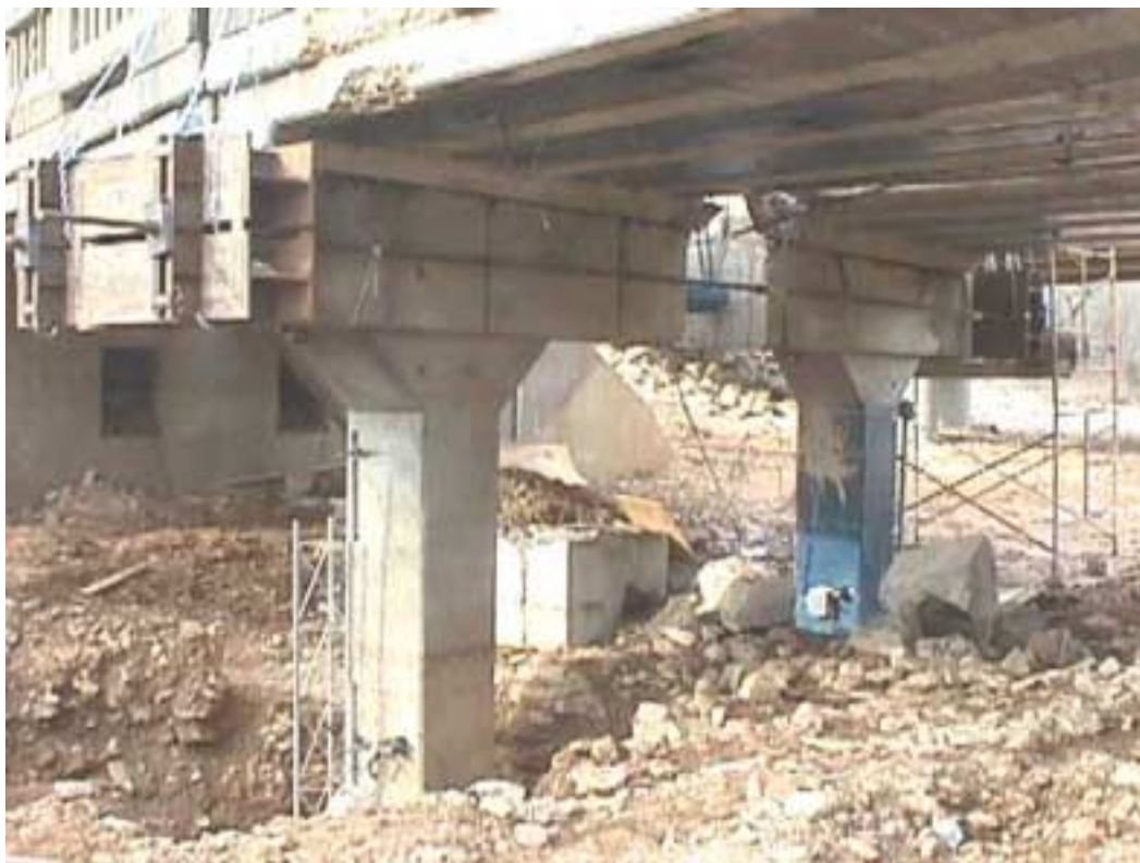
Figure 3.10. Photo showing piers test setup.
