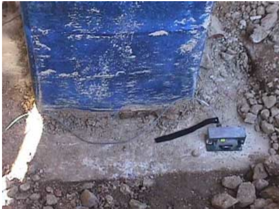
Figure 3.17. Inclinometer on the surface the footing.
