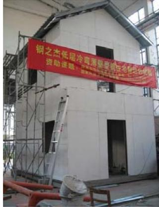
Fig. 1. Shaking table test model
