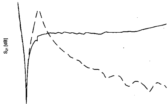
Figure 7. The effect of a distributed capacitor
