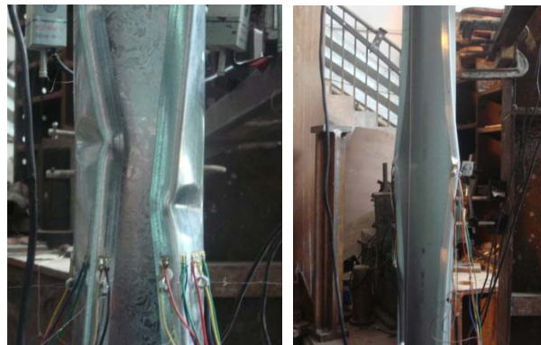
Fig. 5 Failure modes for beam-columns under axial compression and minor axis bending (lips in compression)
