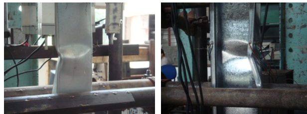
Fig. 3 Failure modes for beam-columns under axial compression and major axis bending
