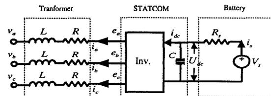
Fig.7 Scheme of a STATCOM with a battery
