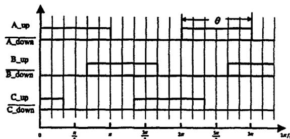
Fig. 1 Switching signals in 180° conduction mode
