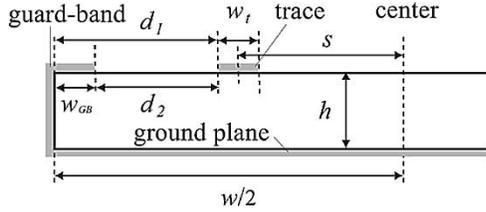
Fig. 11. Cross-section of the PCB showing the relevant dimensions.
