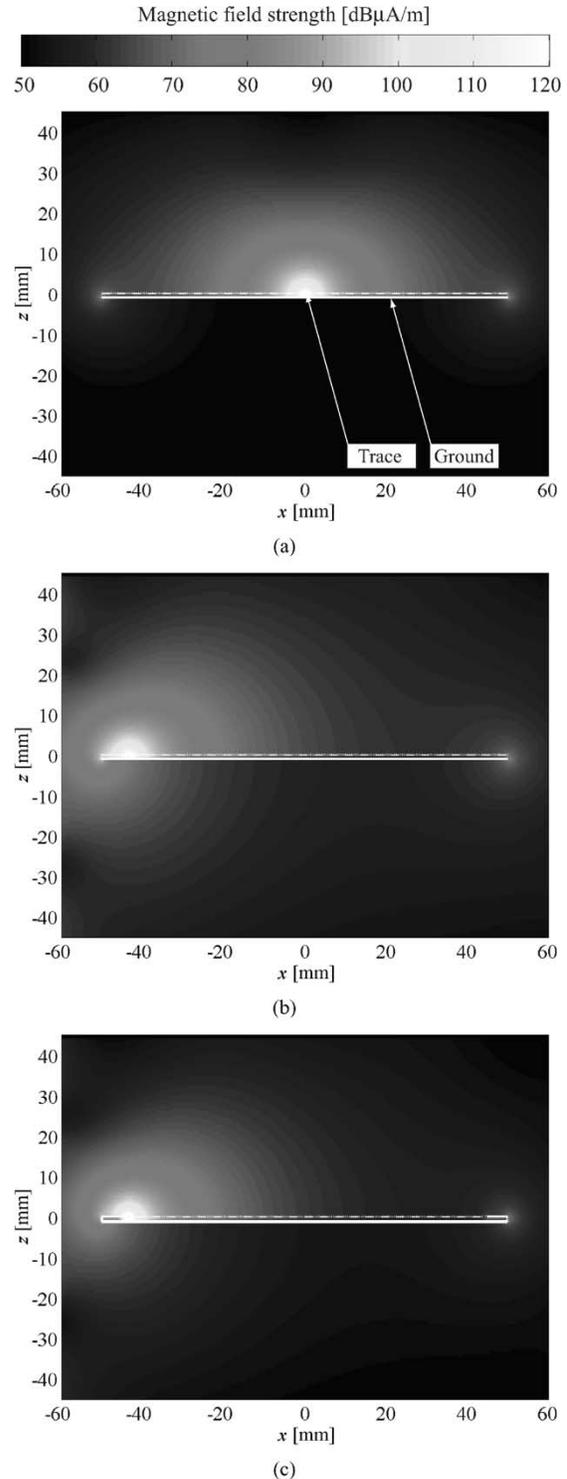
Fig. 9. Magnetic field  $\mathbf{H}$  distribution in the  $x$ - $z$  plane at the center of the PCB. (a) center. (b) d250. (c) d250 GB.
