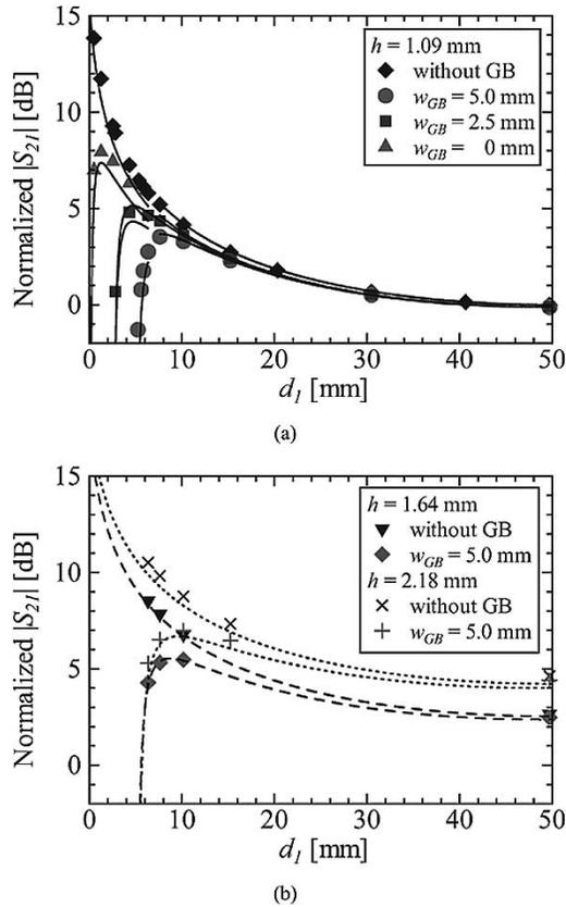
Fig. 14. Normalized  $|S_{21}|$  versus  $d_1$ . Lines are calculated results from (6) and (9), and symbols are FDTD calculated results. (a)  $h = 1.09$  mm. (b)  $h = 1.64$  and  $2.18$  mm.
