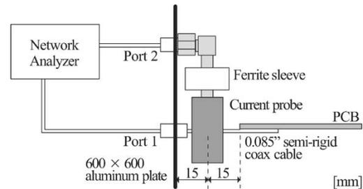
Fig. 3. Experiment setup for CM current measurements.
