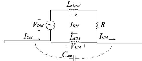
Fig. 1. Equivalent circuit illustrating the current driven mechanism.
