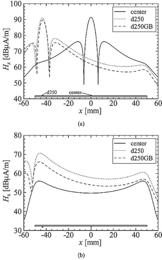
Fig. 10.  $H_x$  distribution along the  $x$  direction. (a) Magnetic field  $H_x$  distribution calculated at 6 mm above the PCB. (b) Magnetic field  $H_x$  distribution calculated at 6 mm under the ground plane.
