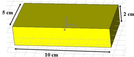
Fig. 1. Empty enclosure surrounded by metal walls.
