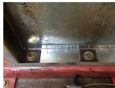
Fig. 8. Shear bolts at bottom of bearing wall
