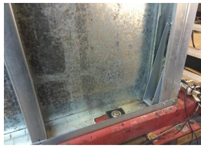
Fig. 6 Hold-down and shear bolts at bottom of shear wall
