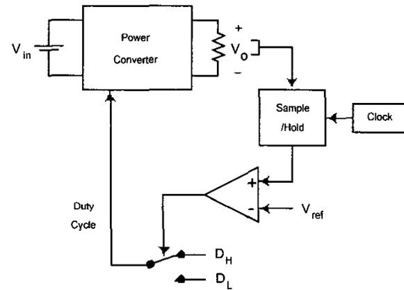
Fig. 17. Block diagram of Pulse Regulation control scheme.
