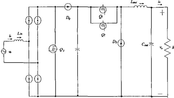
Fig. 4. Boost + interleave buck converter.
