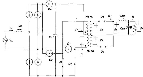
Fig. 9. Mode V ( $Q_1$ : on,  $Q_2$ : off,  $D_3$ : off,  $D_4$ : off).
