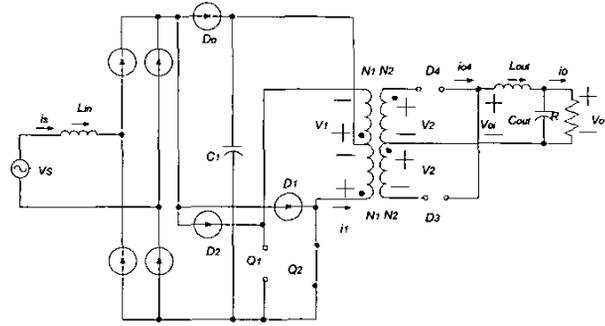
Fig. 8. Mode IV ( $Q_1$ : off,  $Q_2$ : on,  $D_3$ : off,  $D_4$ : off).
