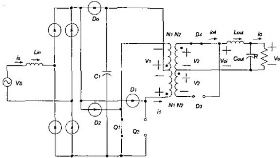
Fig. 7a. Mode I ( $Q_1$ : on,  $Q_2$ : off,  $D_3$ : on,  $D_4$ : off).
