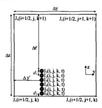
Figure 5. Schematic representation of the FDTD multiwire subcelluar algorithm for the ribbon cable parallel to the x-direction.
