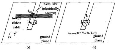
Figure 2. (a) Schematic illustration of the interference physics of the voltage-driven mechanism of the electrically narrow slot; (b) extraction of an EMI antenna impedance through a 3D full-wave model without including the ribbon cables.
