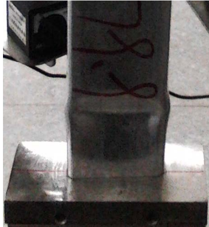
Fig.4 Local buckling mode
