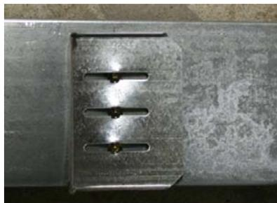
Figure 7: Photo of head-of-wall connector test with extended stud
