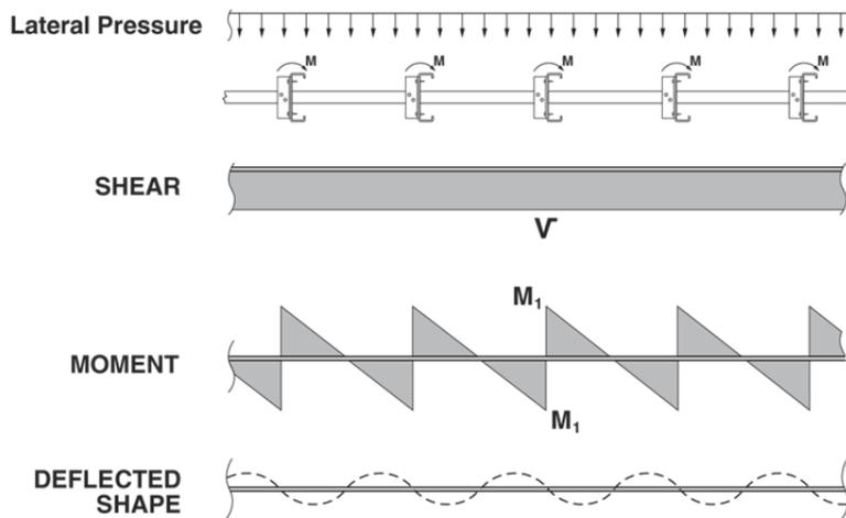
Figure 9: Typical wall system subjected to lateral load
