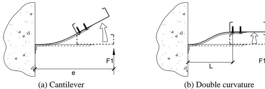
Figure 5: Deformation of bypass connectors resisting in-plane loads
