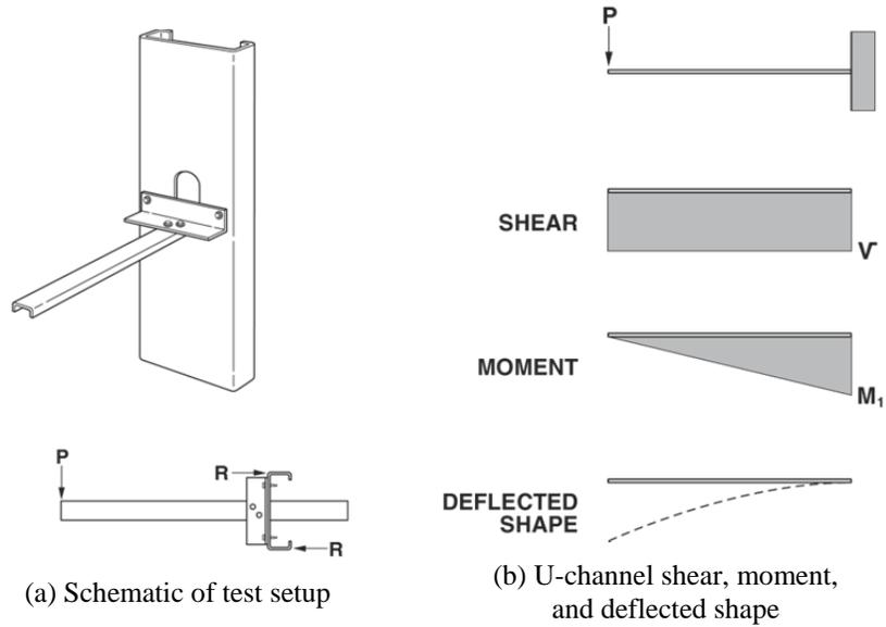
Figure 8: Cantilever test setup for bridging connectors
