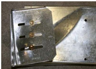
Figure 6: Photo of web failure from head-of-wall connector test
