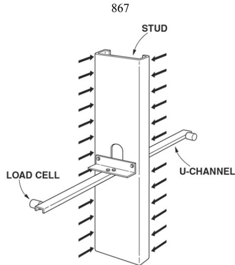
Figure 11: Idealized test setup for bridging connectors
