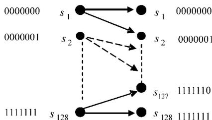
**Fig. 1** Snapshot of the trellis used by BCJR
