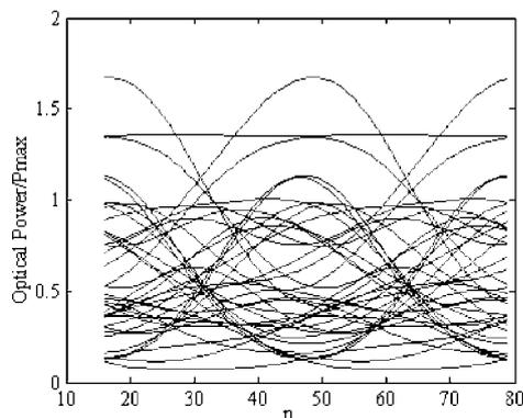
**Fig. 4** Output electrical eye-diagram for  $Q = 3.02$  dB (32 samples/pulse)
