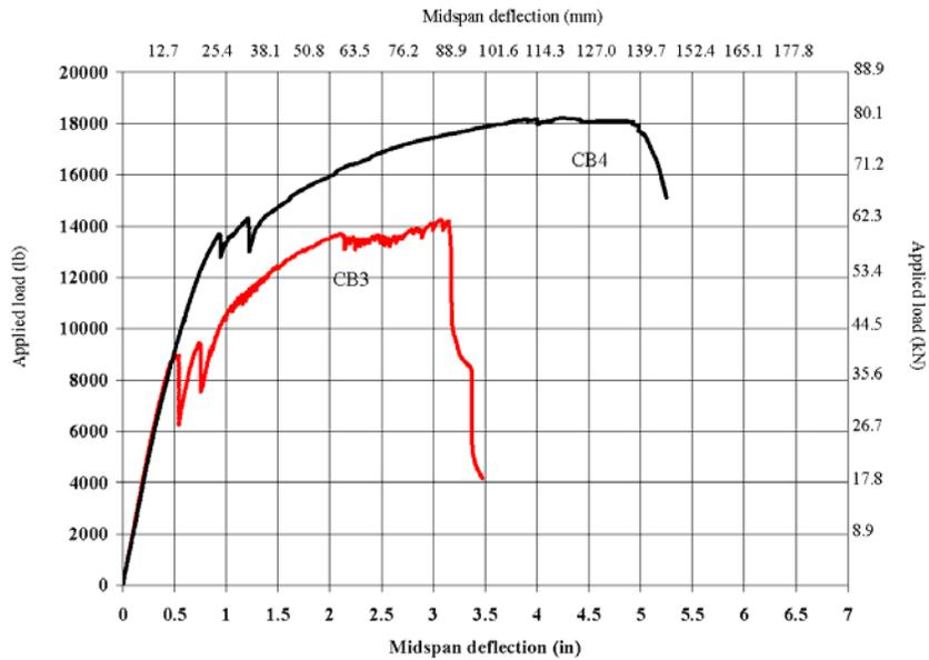
Figure 7 - Applied loads versus mid-span deflection curve for Specimens CB3 and CB4
