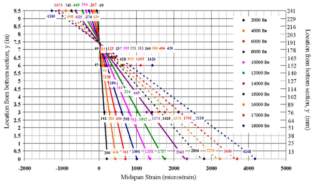
Figure 9 - Applied loads versus strain distribution at midspan for composite section CB4
