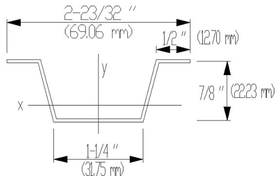
**Figure 4** - Furring channel section
