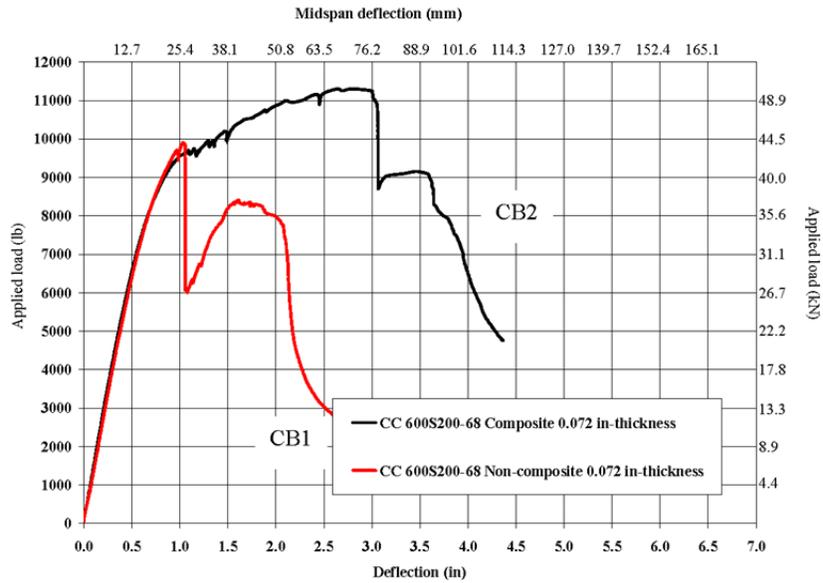
Figure 6 - Applied loads versus mid-span deflection curve for Specimens CB1 and CB2
