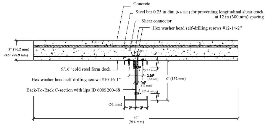
**Figure 2** - Composite section and details of connection (Specimens CB2, CB4 and CB5)
