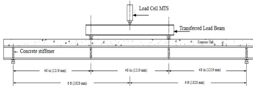
**Figure 5** - Four-point bending test setup
