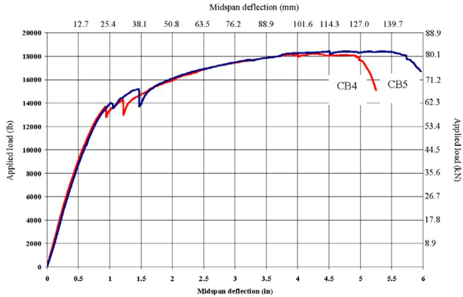
Figure 8 - Applied loads versus mid-span deflection curve for Specimens CB4 and CB5
