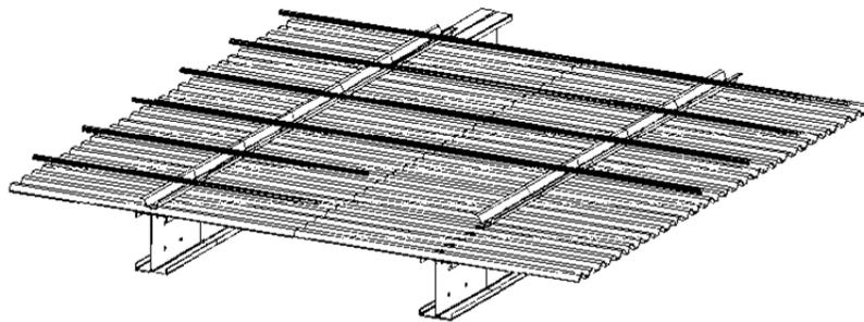
**Figure 1** – Composite beam system before casting
