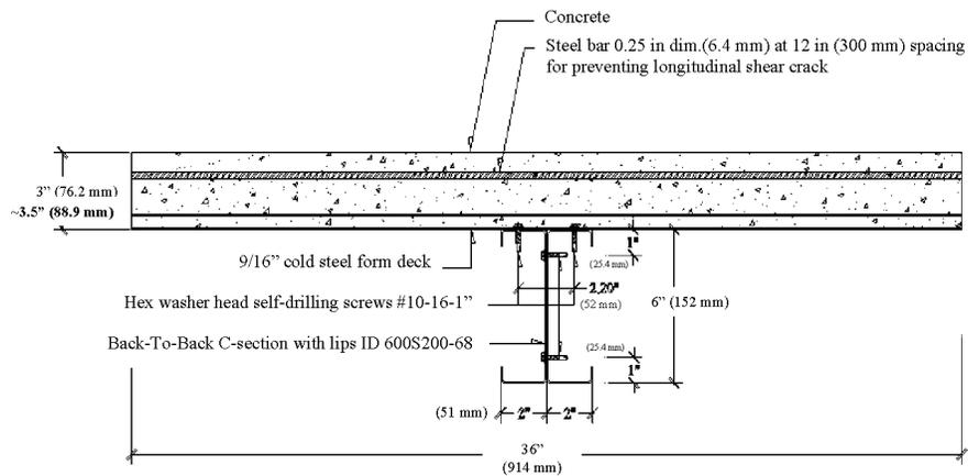
**Figure 3** - Non-composite section and details of connection (Specimens CB1 and CB3)
