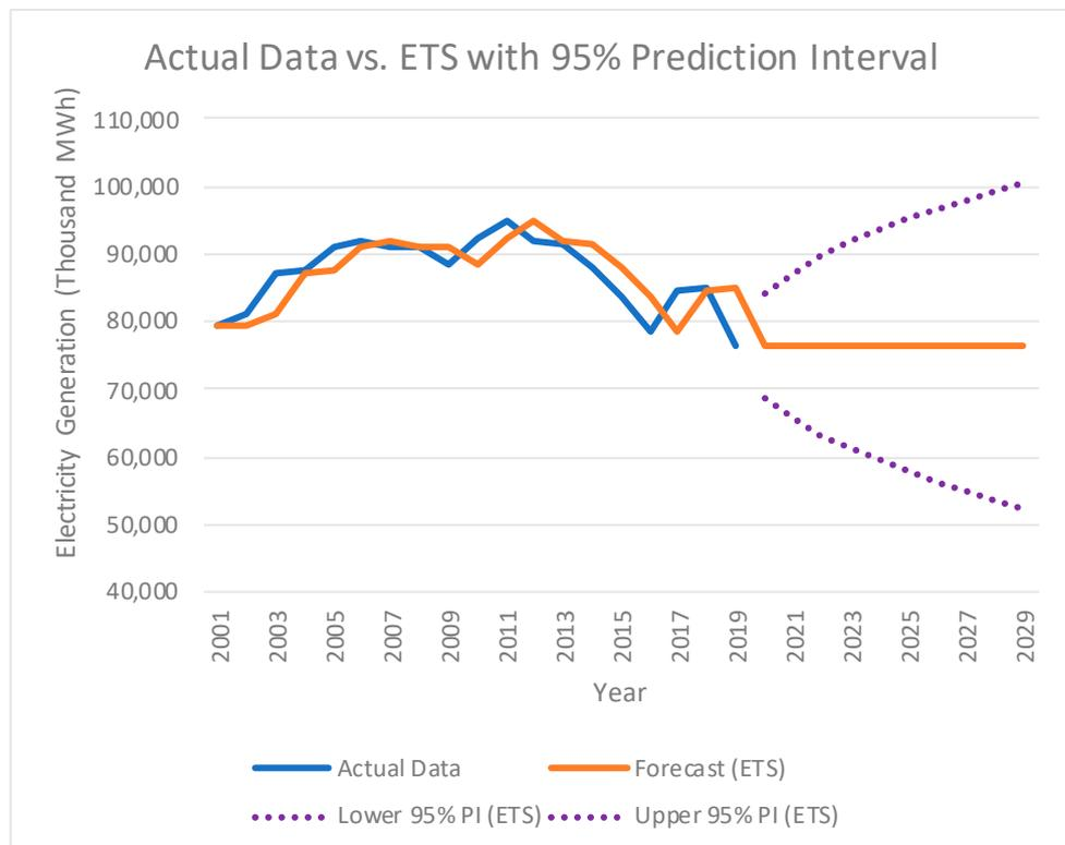
Figure 4. Actual Data vs. exponential triple smoothing (ETS) with 95% Prediction Interval.
