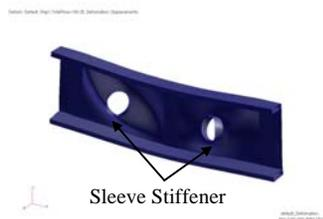
Figure 10: Shear Failure Mode of 200x45x1.6 LSB with 60 mm Web Openings and 20 mm Sleeve Stiffeners
