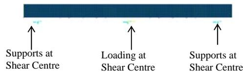
(b) Applied Loads and Boundary Conditions (Plan View)
