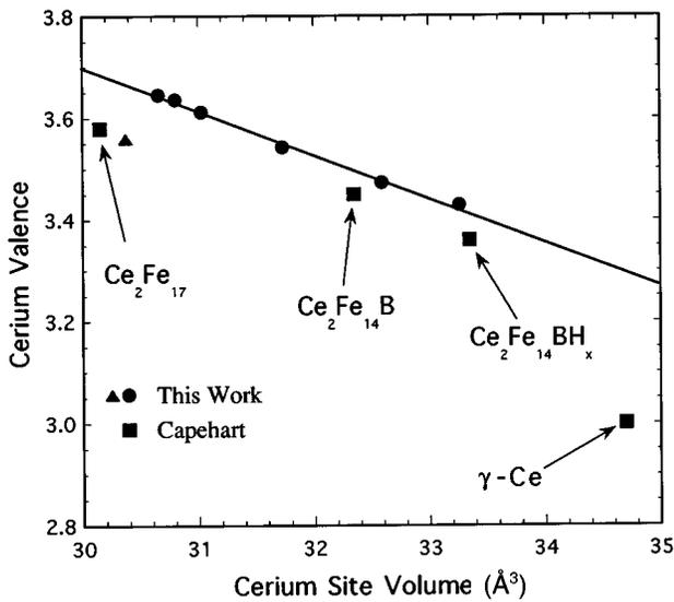
FIG. 3. The cerium spectroscopic valence versus the cerium site volume in  $\text{Ce}_2\text{Fe}_{17-x}\text{Al}_x$ ,  $\bullet$ ,  $\text{Ce}_2\text{Fe}_{14}\text{Si}_3$ ,  $\blacktriangle$ , and in  $\text{Ce}_2\text{Fe}_{17}$ ,  $\text{Ce}_2\text{Fe}_{14}\text{B}$ ,  $\text{Ce}_2\text{Fe}_{14}\text{BH}_x$ , and  $\gamma$  cerium. The  $\blacksquare$  data points were obtained from Ref. 2.
