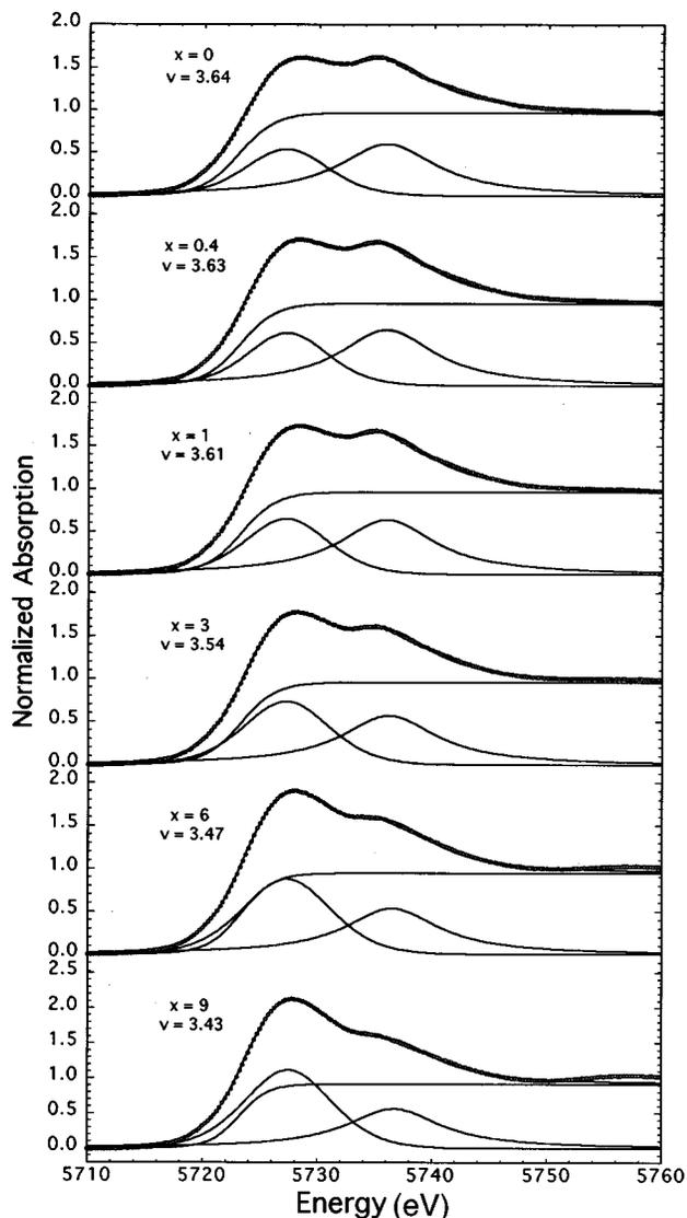
FIG. 1. Cerium  $L_{III}$ -edge XANES spectra of  $Ce_2Fe_{17-x}Al_x$ , where  $x$  is 0, 0.4, 1, 3, 6, and 9. The fits shown are model  $d$  described in the text.
