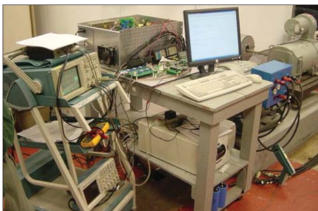
FIGURE 6 Laboratory setup of a typical ship power system for CI based design of an optimal excitation controller.
