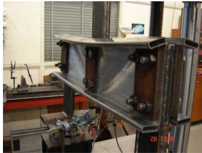
Figure 8: Elastic Shear Buckling
