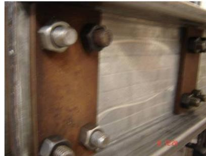
Figure 9: Inelastic Shear Buckling
