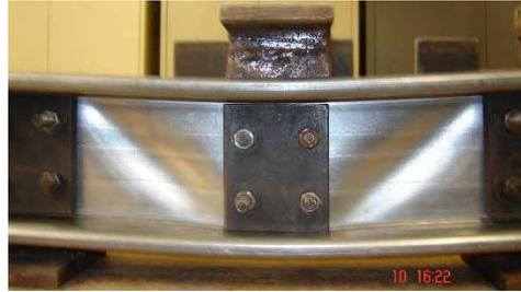
Figure 7: Shear Yielding Failure
