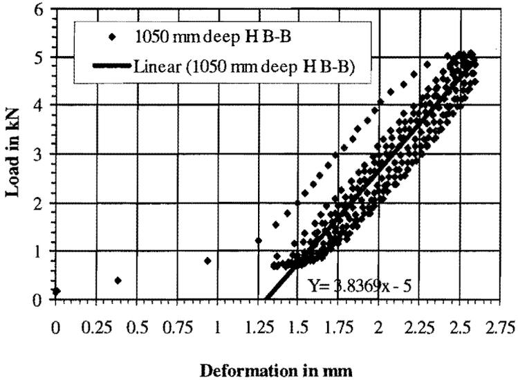
**Fig. 6: A typical load-deformation curve**
