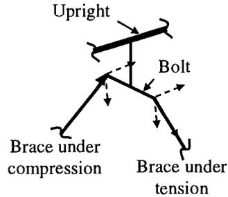
**Fig. 8: Forces at a joint**
