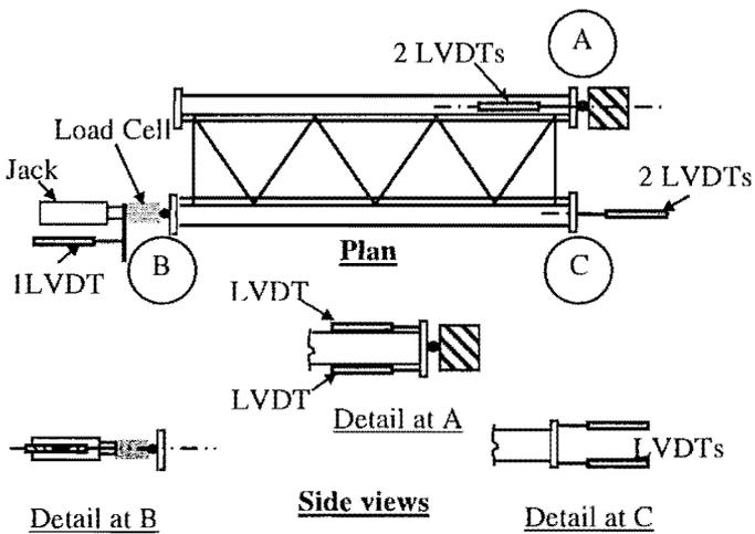
**Fig. 5: Test set-up and LVDT locations**
