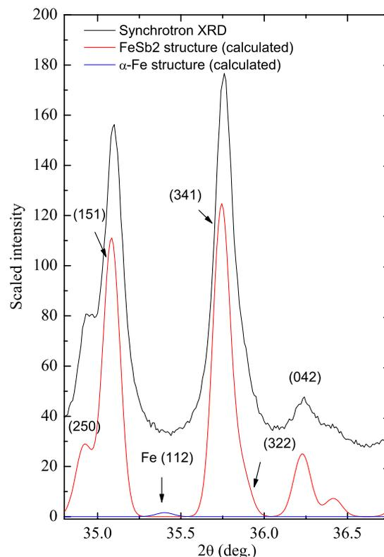
FIG. 6. (Color online) Observed (black) and calculated (red) synchrotron powder x-ray diffraction patterns of  $\text{Fe}_{0.75}\text{Co}_{0.25}\text{Sb}_2$ . Calculated pattern includes 0.3% of a superimposed  $\alpha$ -Fe impurity. If present, the impurity would have caused detectable deviation of the observed pattern since there is no peak overlap.
