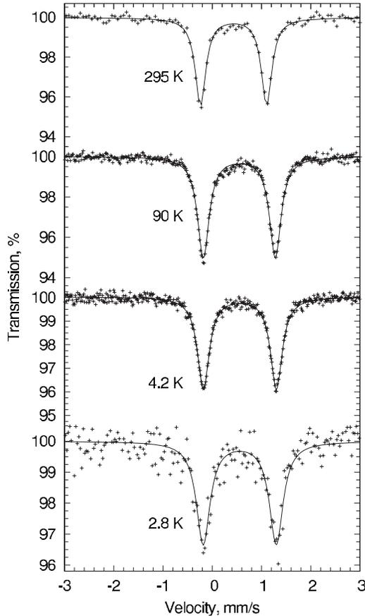
FIG. 3. The  $^{57}\text{Fe}$  Mössbauer spectra of  $\text{Fe}_{0.75}\text{Co}_{0.25}\text{Sb}_2$  at the indicated temperatures. The solid line is a fit to a doublet, using the parameters indicated in Table I.
