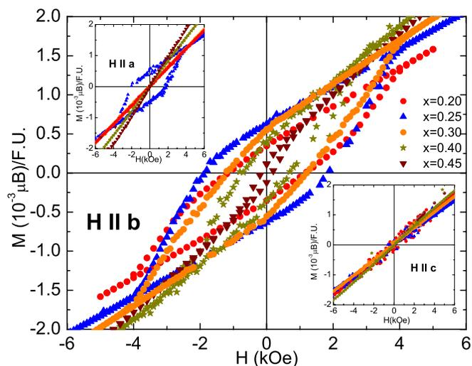
FIG. 2. (Color online) Hysteresis loops for  $\text{Fe}_{1-x}\text{Co}_x\text{Sb}_2$  in the ferromagnetic state ( $x=0.2-0.45$ ) at  $T=1.8$  K. Magnetization does not saturate; it continues to increase with applied magnetic field, similar to bulk itinerant ferromagnets with  $3d$  ions.
