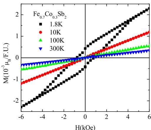
FIG. 5. (Color online) Magnetic hysteresis for the  $\text{Fe}_{0.7}\text{Co}_{0.3}\text{Sb}_2$  sample. It is important to note the absence of hysteresis loops above the ferromagnetic transition of  $\text{FeSb}_2$ . Data were taken on a crystal from independently grown batch.
