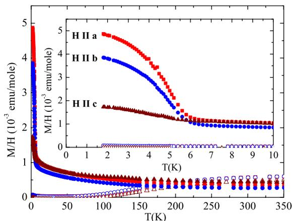
FIG. 1. (Color online) Magnetic susceptibility  $M/H$  of  $\text{FeSb}_2$  (open symbols) and  $\text{Fe}_{0.75}\text{Co}_{0.25}\text{Sb}_2$  (solid symbols) for a 1-kOe field applied along all three principal crystalline axes.
