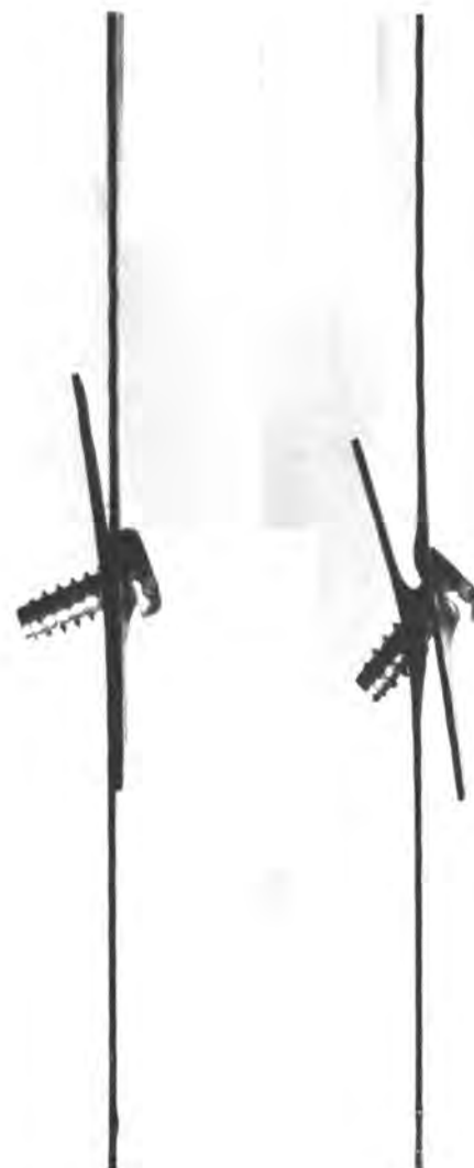
Test on a screwed connection Failure mode : inclination of fastener
