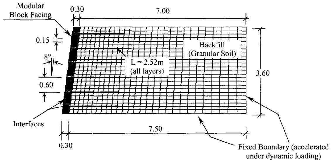
Fig. 1 Discretised model of segmental (modular block) retaining wall system at end of construction (dimensions are in metres).
