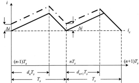
**Figure 2.** Valley current control under trailing edge modulation.
