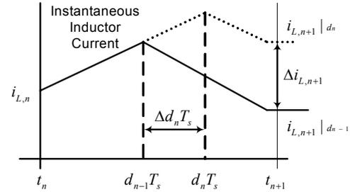
Figure 8. Inductor current during one switching period.
