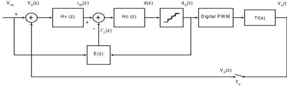
Figure 6. Sensor less current mode control scheme.
