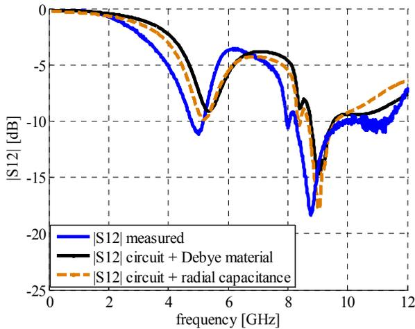
Figure 11. Effect on  $|S_{12}|$  of radial capacitance term
