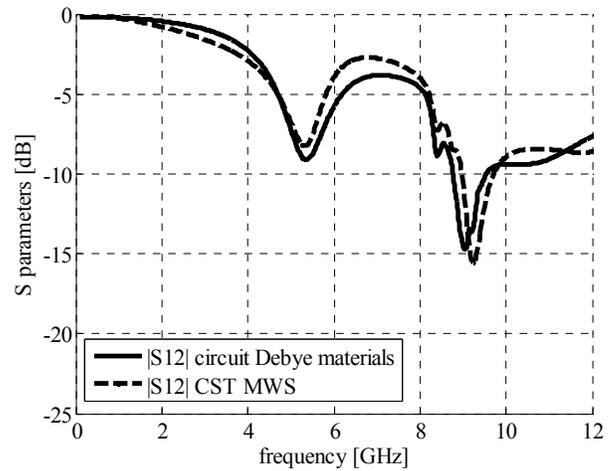
Figure 9.  $|S_{12}|$  Microwave Studio vs. circuit model
