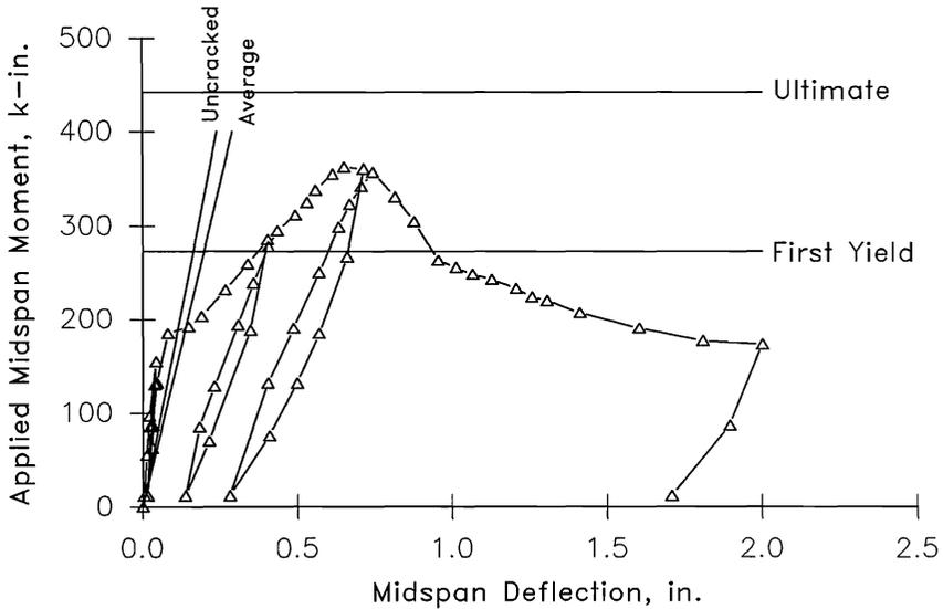
**Figure 4.** Applied Midspan Moment vs. Midspan Deflection : SDI-2-1
