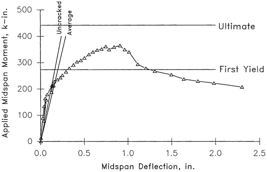
Figure 5. Applied Midspan Moment vs. Midspan Deflection : SDI-2-2
