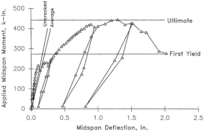
Figure 7. Applied Midspan Moment vs. Midspan Deflection : SDI-4-1
