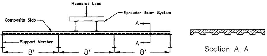
**Figure 1.** Schematic of Test Setup (center span test)
