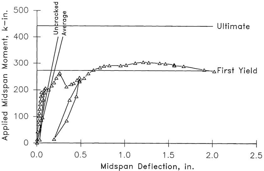
Figure 8. Applied Midspan Moment vs. Midspan Deflection : SDI-4-2
