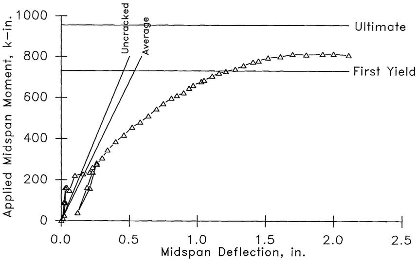
Figure 6. Applied Midspan Moment vs. Midspan Deflection : SDI-3-1
