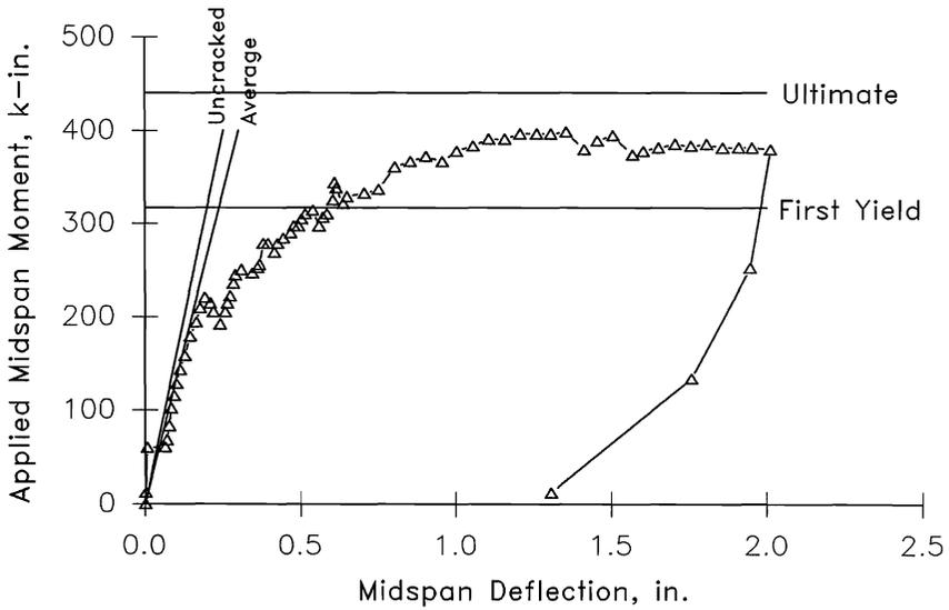
**Figure 3.** Applied Midspan Moment vs. Midspan Deflection : SDI-1-1
